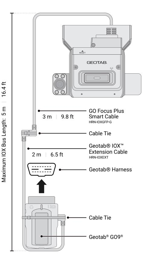
The Geotab GO 9 has a rich ecosystem of IOX Add-Ons. The GO Focus Plus supports IOX Add-Ons on the IOX BUS with the following conditions:
