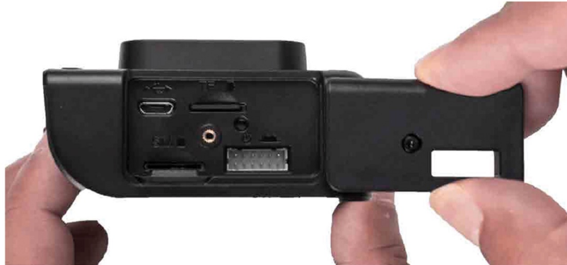
Removing the right panel I/O cover
