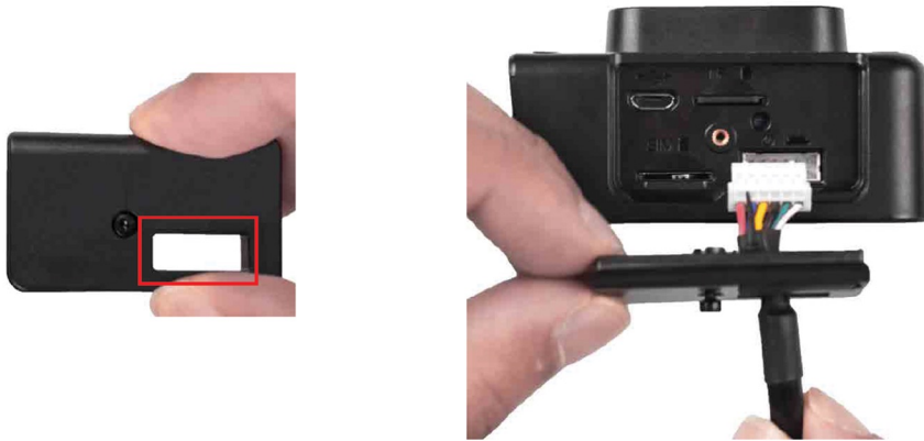
Feeding the 12-pin connector cable through the hole on the I/O cover
