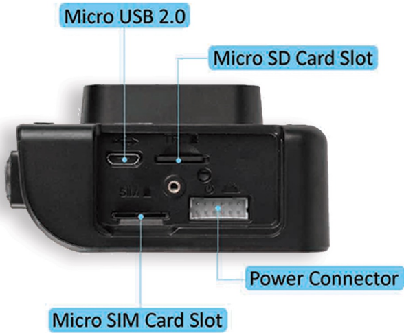
Figure 4: Right panel I/O layout
