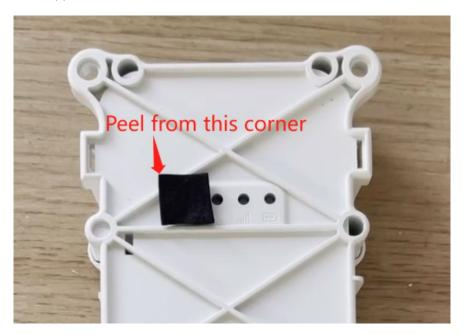
2. Make sure the round foam stays on the device, only peel off the square foam.
