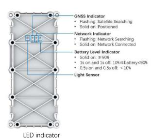
Note: Indicator lights will go out automatically after the tracker turns on for 70 seconds without connecting to the external power via USB cable.
