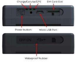
On/Off Switch: Used to turn the device on and off.
